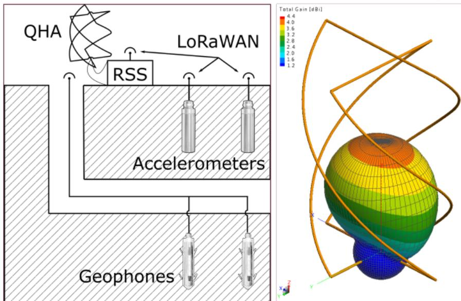
Figure 7: Remote Sensing Station Setup
