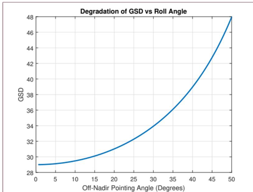
Figure 10: Imager GSD vs Roll Angle
