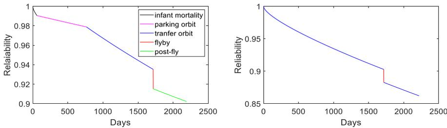
**Figure 5: Reliability dividing the mission in different phases (left) and considering all subsystems active (right).**
