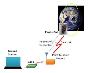
Figure-2 PARDUS-SAT system that is composed of a space segment and a ground segment
