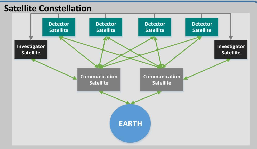
Figure 2: Satellite Constellation Satellite constellation will be consisted of 8 satellites with 3 group:
