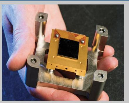
Figure 6: NEOCam Sensor <sup>4</sup>
