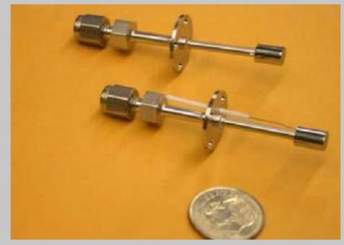
Figure 4: Miniature Xenon ION (MiXI) thruster <sup>2</sup> Figure 5: MiXI's Miniature Hollow Cathodes <sup>3</sup>
