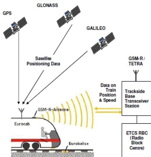
Figure 3 General scheme for ETCS using the GPS or Galileo Satellite constellation for positioning<sup>4</sup>.
