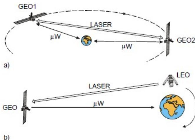
Fig. 5 Two geostationary satellites (GEO1, GEO2) are connected by a laser duplex link (a). A low-earth orbiting satellite (LEO) transmits data via a laser link to a GEO acting as data relay (b). In both cases the downlink is via microwaves ( $\mu\text{W}$ ).<sup>5</sup>
