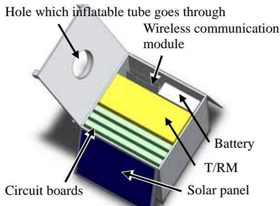
Figure 5 Inner structure of power transmitting satellite.
