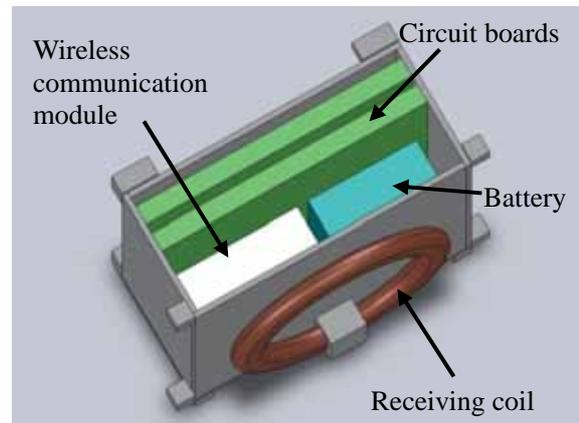
Figure 6 Inner structure of receiving satellite.
