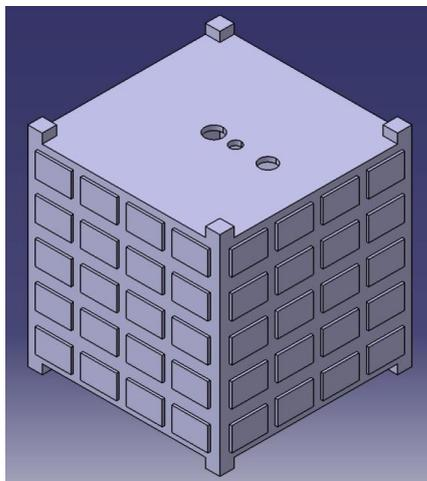
Figure 2: Main Satellite of the each formation flight (It acts of both transmitter and receiver, is a cube of  $40 \times 40 \times 40 \text{ cm}^3$ ).
